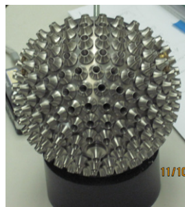
RadBall™ is a radiation-mapping device that can be deployed into high dose fields and operated remotely to characterize gamma-ray radiation sources.
