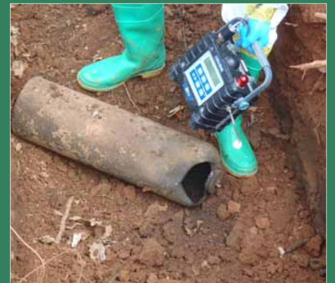
An AreaRae, which is a specialized gas meter, was used post explosion to detect if all of the toxic product had burned off in the blast, March 8, 2011.
