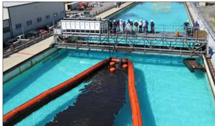
Oil recovery efficiency is calculated in a test tank using real oil spilled into differing sea conditions at the Ohmsett training facility in Leonardo, N.J., May 10, 2011. U.S. Coast Guard photo by Dale Hemenway.
