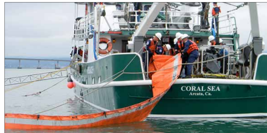
Coast Guard pollution responders from the Marine Safety Detachment Humboldt Bay and the Pacific Strike Team deploy and work with a Vessel of Opportunity Skimming System aboard the research vessel Coral Sea, June 21, 2011. U.S. Coast Guard photo by Seaman Erika Lindquist.
