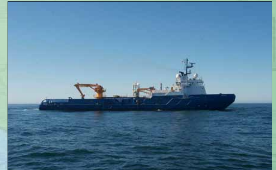
The Nanuq, a 301-foot oil spill response vessel that has been outfitted to deploy an underwater remotely operated vehicle, sits six and a half miles off the coast of Cambria, Calif. U.S. Coast Guard photo by Petty Officer 3rd Class Cory Mendenhall.
