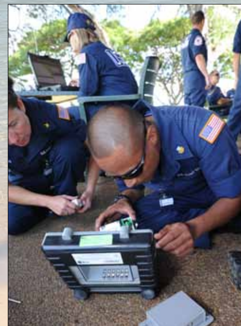
Petty Officer 1st Class Truman Skang with the PST replaces the sensors inside the AreaRae detector, Nov. 8, 2011.
