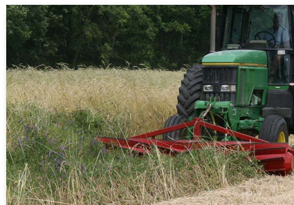
Termination of vetch and rye cover crop using a curved bar roller crimper
