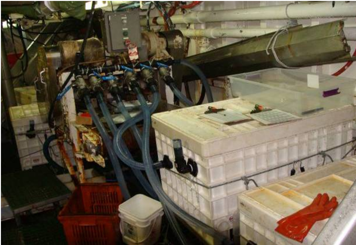
Figure 2. Halibut holding tanks and water supply manifold.
