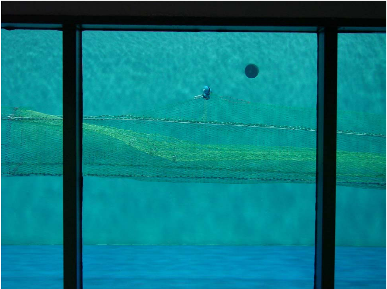
Figure 7: Final design product for an improved flapper excluder from fall 2009 flume tank work
