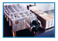
Monitor (SUSIM) which measured absolute solar UV irradiance and examined the impact of solar variability on the Earth's ionosphere and climate. SUSIM also flew on the Upper Atmosphere Research Satellite (UARS) (1991-2005) and produced the longest continuous absolute measurement of solar UV irradiance to date.
