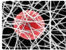
eSpin Technologies' SBIR contract was used to develop nanofibers for air filters to stop particulates smaller than 3 microns
