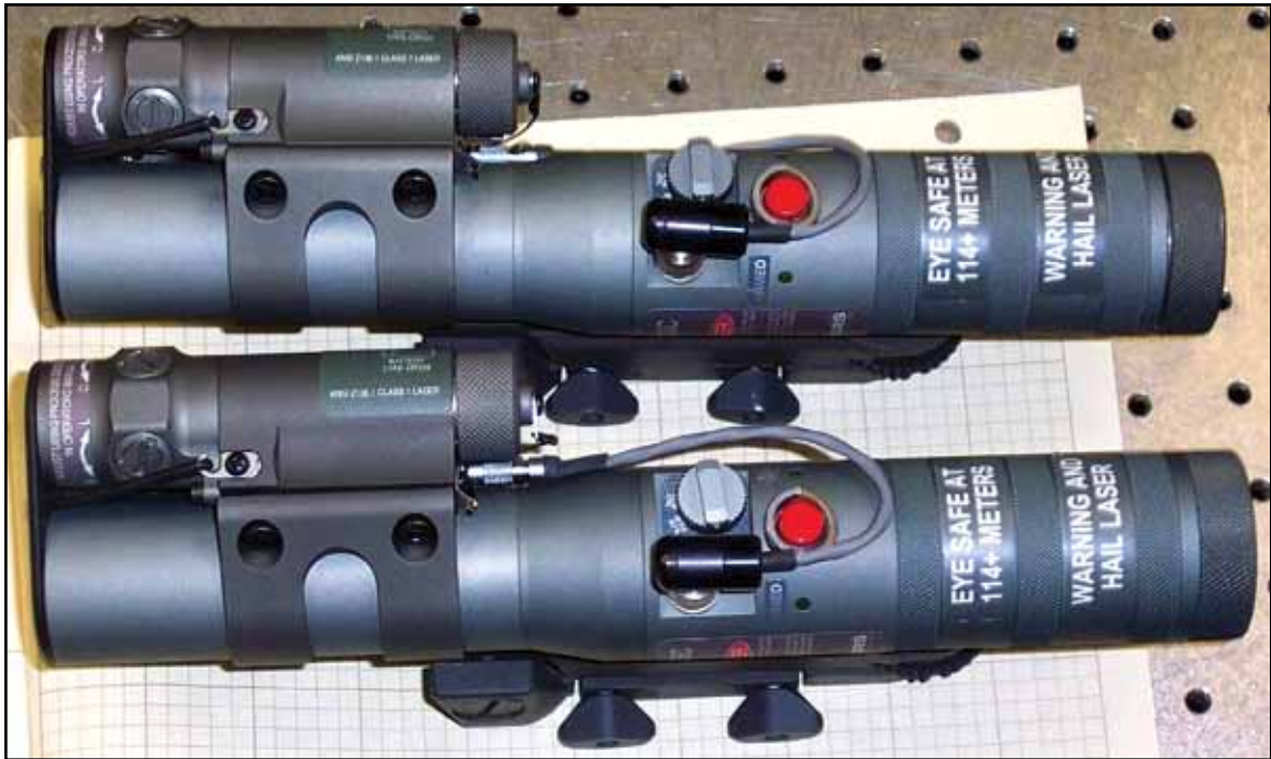
Figure 3. GBD-IIIC Dazzling Laser System Under Evaluation
