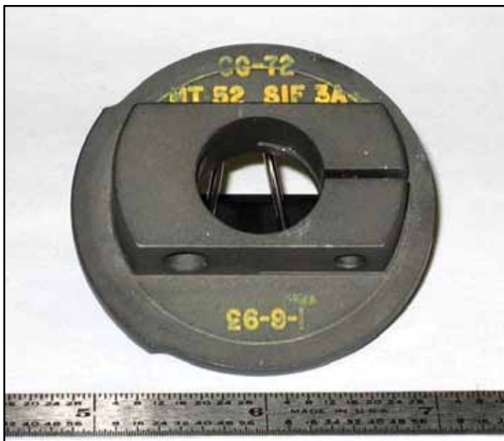
Figure 1. MK 45 Gun FCO Cam
