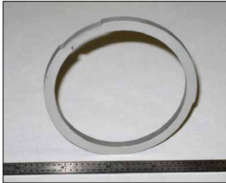
Figure 3. 76mm Gun FCO Cam
