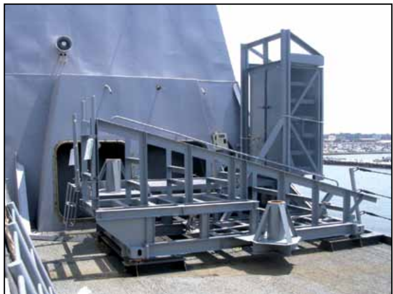
Figure 1. Shipboard MOGAS Rack Storage System
