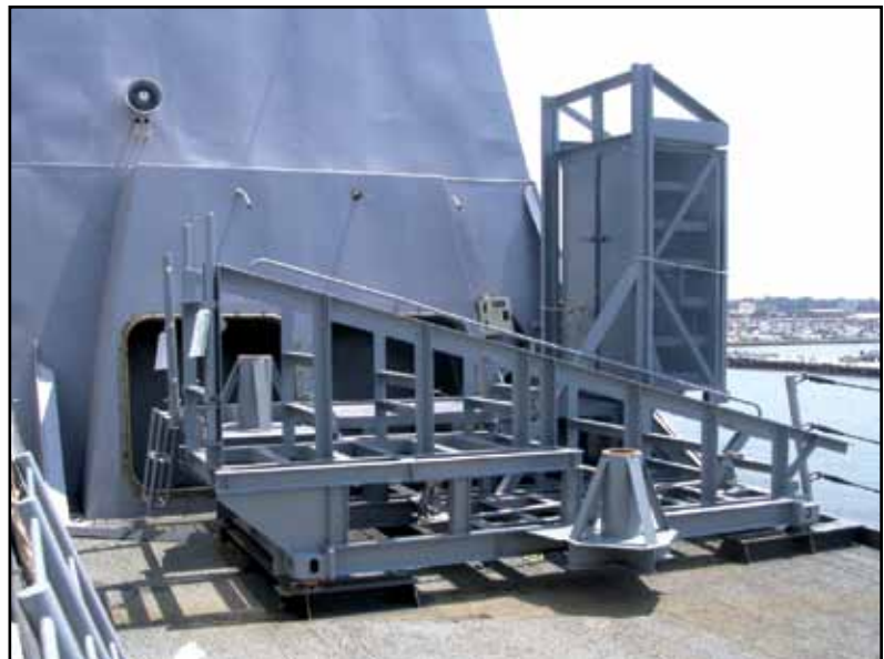
Figure 1. Shipboard MOGAS Rack Storage System
