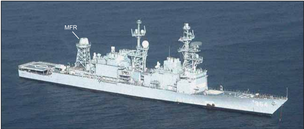
Figure 1. AN/SPY-3 Multifunction Radar (MFR) Installed on SDTS
