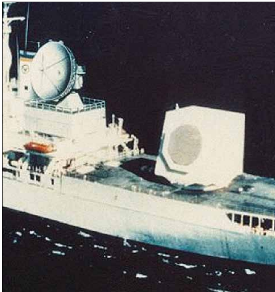
Figure 2. Close-Up of Cobra Judy S-Band Phased Array and X-Band Dish Antenna
