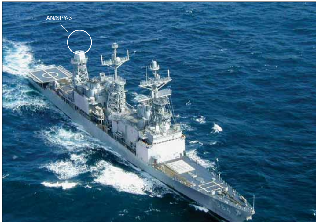
Figure 4. AN/SPY-3 Self-Defense Test Ship Installation
