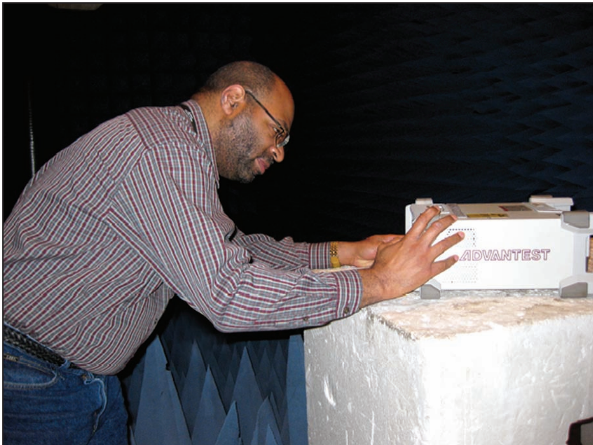
Figure 3. An NSWC Dahlgren employee adjusts a spectrum analyzer—a tool used to perform a typical spectrum certification measurement.
