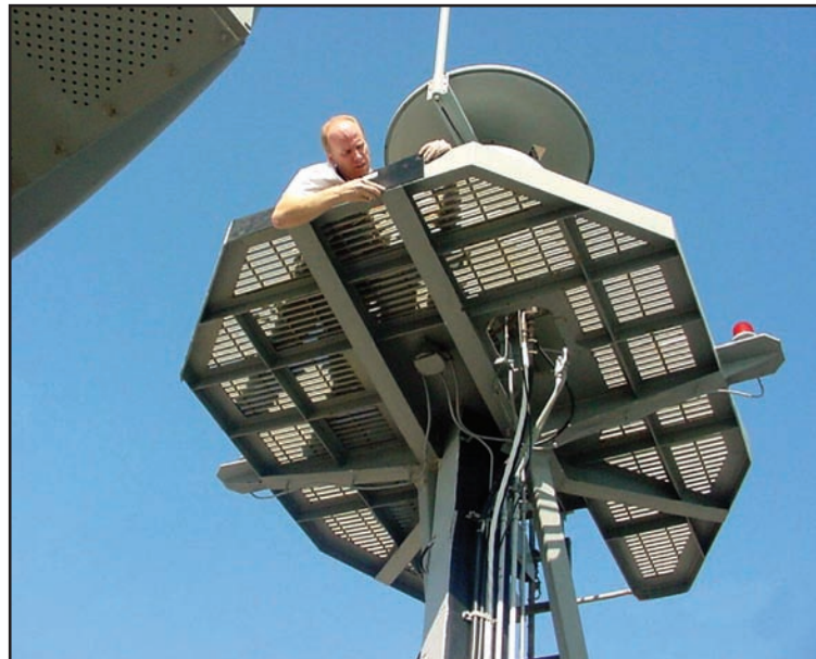
Figure 2. X-Band RAM Installation on USS Ronald Reagan (CVN 76) Stubmast Showing New (Black) Tile
