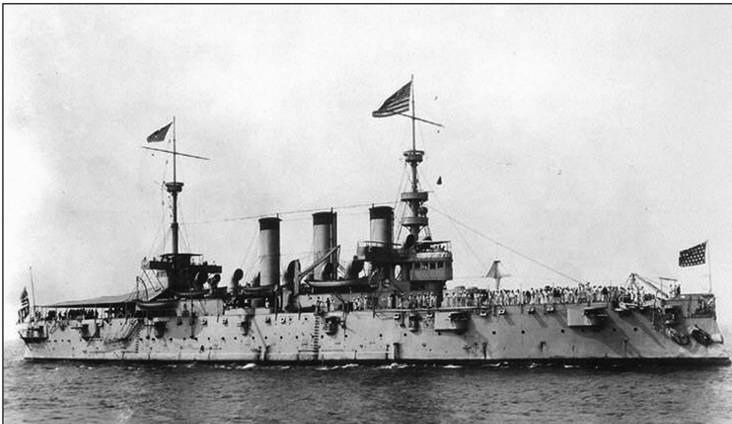
Figure 1. USS New York (CA 2) taken in the Summer of 1898. The wireless system's antenna ran from a wooden mast mounted on the topmast to the after gun room. (Navy Historical Center Photograph)
