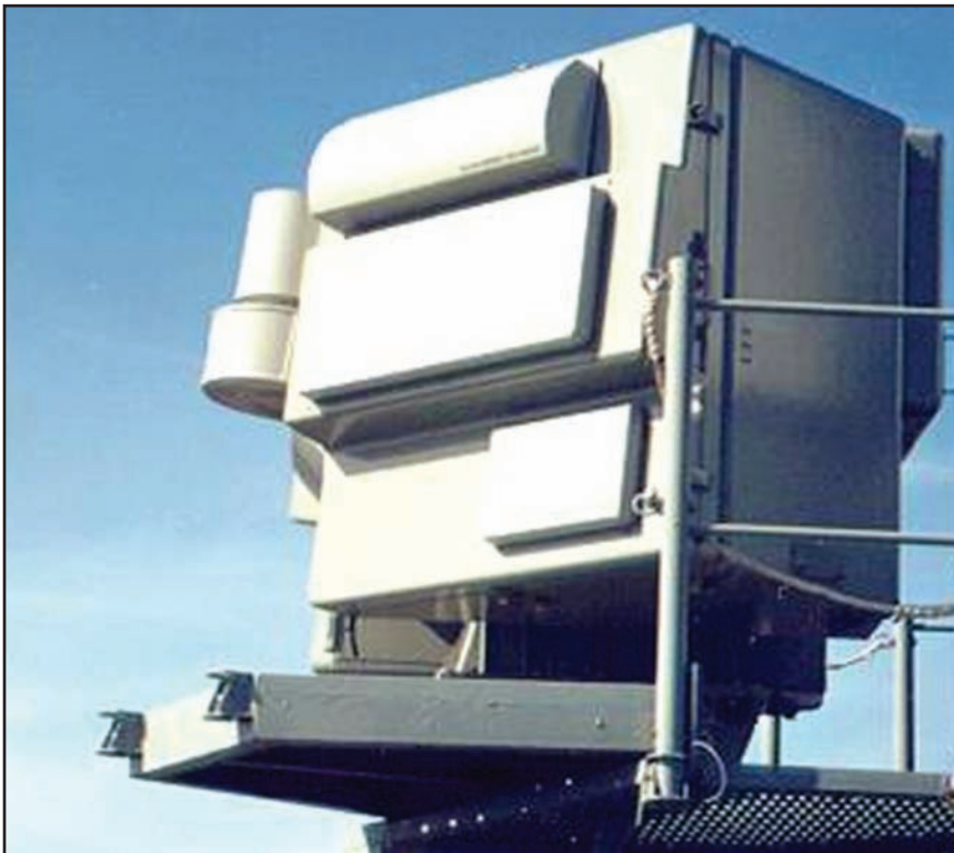
Figure 2. AN/SLQ-32 Antenna Enclosure
