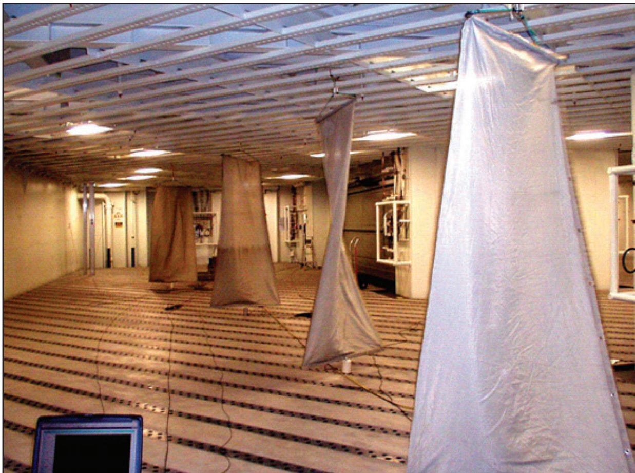
Figure 3. Energy Stirring Using Tuner Assemblies Aboard USNS Sacagawea (T-AKE 2)
