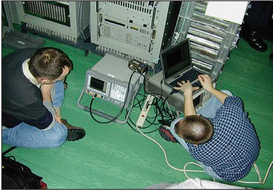
Figure 2. Two EMC Engineers Analyze Spectrum Characteristics to Solve an EMI Problem
