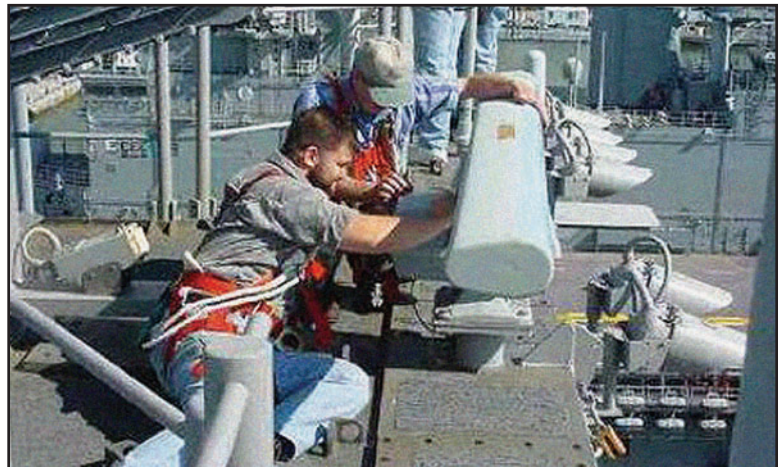
Figure 5. EMI Problem Solvers Troubleshoot a Navigation Radar
