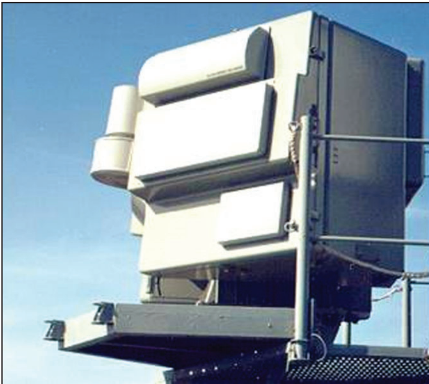
Figure 2. AN/SLQ-32 Antenna Enclosure
