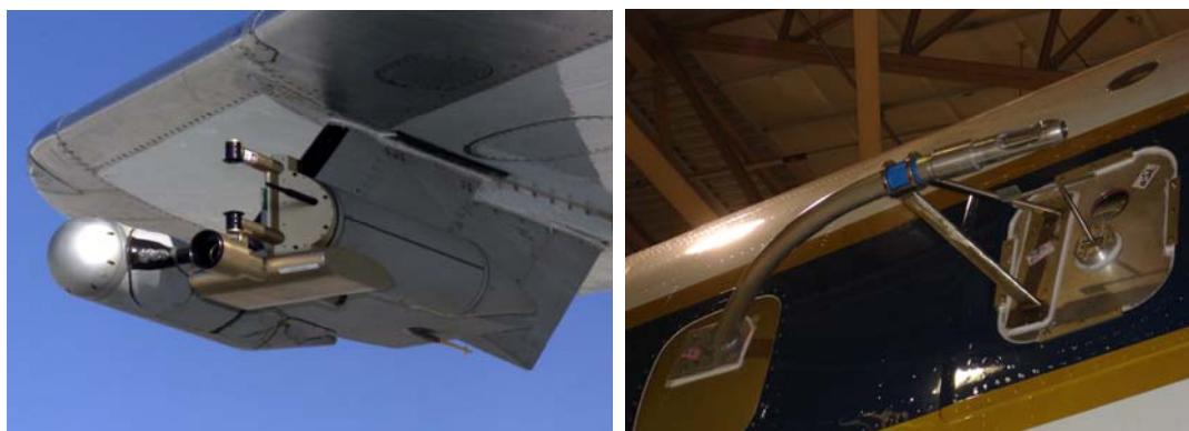
Figure 1. Wingtip-mounted Cloud Aerosol and Precipitation Spectrometer (CAPS, left) and the window-mounted iso-kinetic aerosol inlet (right) used to supply sample air to the LARGE instrument rack.
