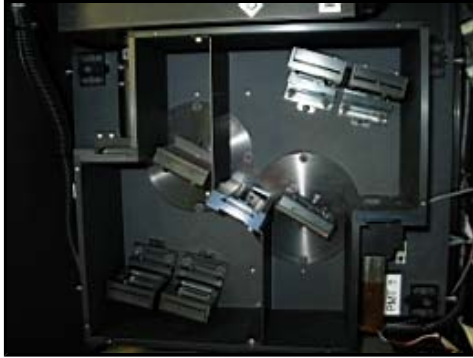
Double monochromator of the SUV-150B spectroradiometer
