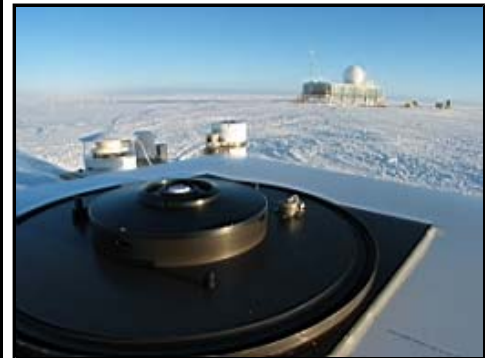
Entrance optics of SUV-150B (foreground) a PSP pyranometer and GUV-511 multi-filter radiometer (middle ground) and the "Big House" at Summit (background)
