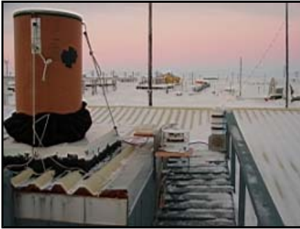
Calibration of the SUV-100. The brown barrel protects the calibration from ambient light.
