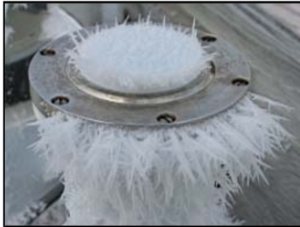
Hoar frost on a PSP pyranometer.
