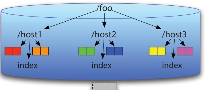
PLFS container for typical parallel file system. Contains a sub-directory per host, each containing an index file and a data log per writer. These files may grow throughout the lifetime of
