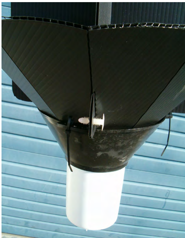
Figure 4-3 Example of Collection Cup of Cross-vane Panel Trap
