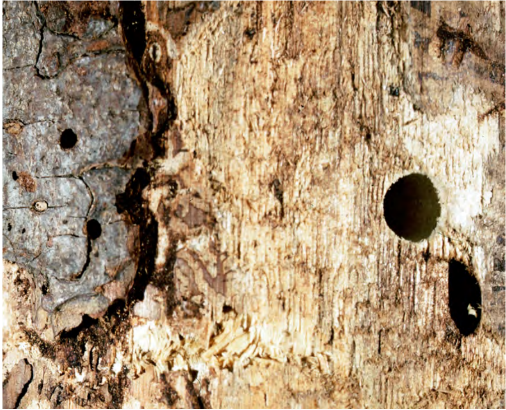
Figure 4-12 Larva Entrance Hole (right) and Adult Exit Hole (left) for Monochamus sutor Linnaeus (Cerambycidae) (Stanislaw Kinelski, http://www.bugwood.org UGA 1258226)
