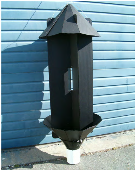
Figure 4-2 Example of Cross-vane Panel Trap
