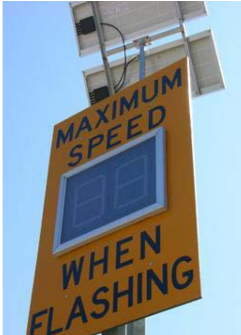
Figure 2. Example of Variable Speed Advisory Sign (Source: Maine DOT)
