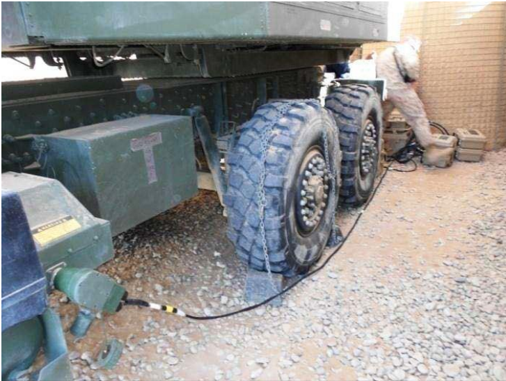
Figure 19 Vehicle Battery Box
