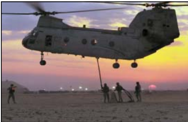
Marines from Service Support Group 15 connect an external load to a CH-46E helicopter during training at Udairi Range, Kuwait. Feb. 18, 2005. Photographer: Lance Cpl. Thomas J. Grove. (Third U.S. Army Public Affairs)
