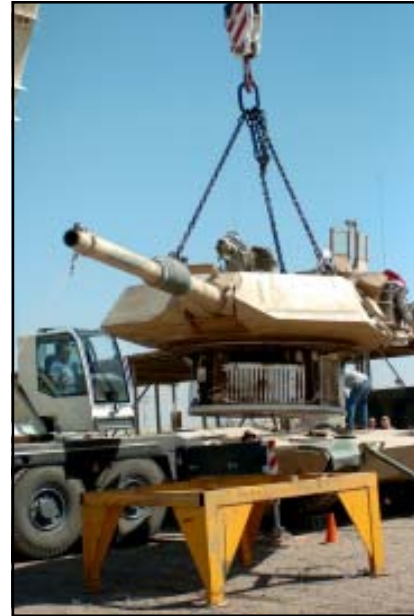
(At right) Civilian workers of the Maintenance Support Team, 1 st Battalion, 13 th Armored Regiment, 3 rd Brigade, 1 st Armored Division remove a M1A1 tank turret to work on the tank's interior. Oct. 13, 2005. Photographer: SOC Matthew Wester. (DVIDS 10988)
