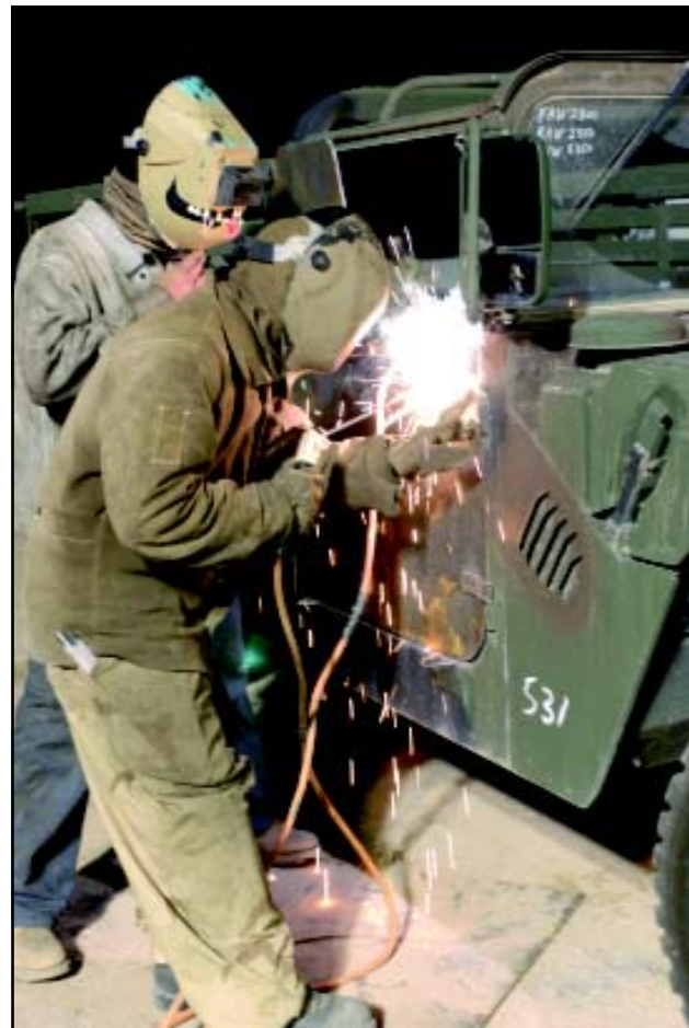
Two Department of Defense contractors weld defensive armor plate to a HUMVEE in Kuwait. No date. (Third U.S. Army Public Affairs)
