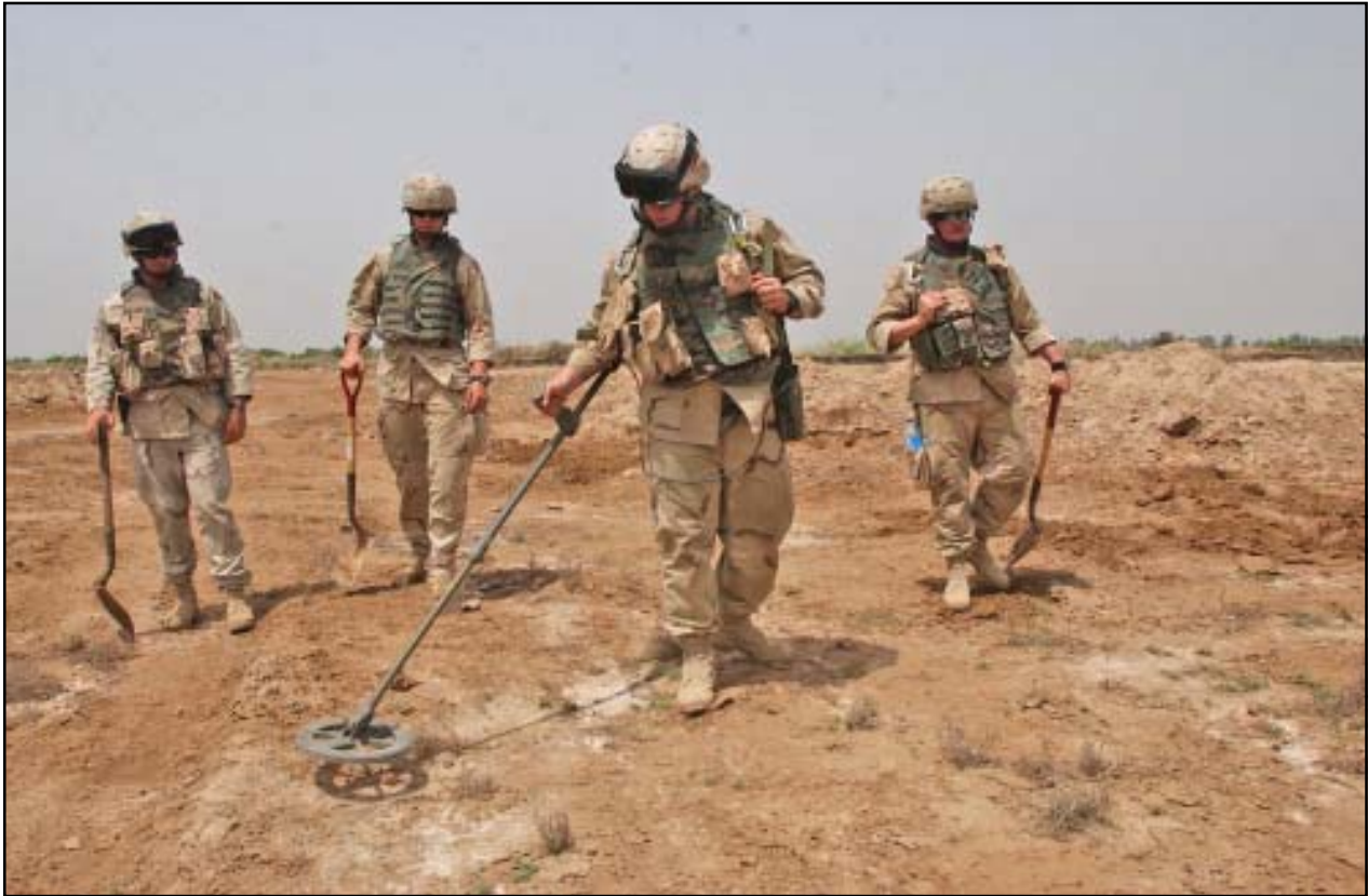
Combat engineer Soldiers from the 3 rd Battalion, 69 th Armor Regiment use a mine detector to search for buried unexploded ordnance at the Tarmiyah Poultry Farm near Balad, Iraq. May 13, 2005. Photographer: SGT Daniel W. Bailey. (DVIDS 6111)
