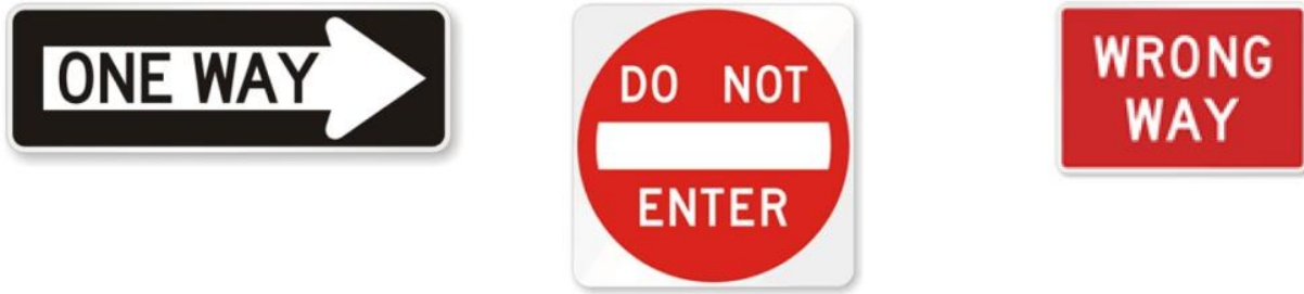
Figure 14. Three signs required, as a minimum, at exit ramps intersecting with a crossroad (from left to right: R6-1 One Way, R5-1 Do Not Enter, R5a-1 Wrong Way).
