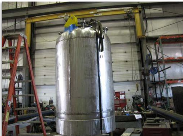
Sludge Transportation Storage Cask Test Article
