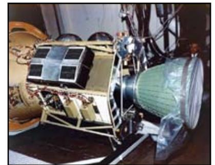
TIMATION I (rectangular object in center of photo) was successfully tested in a "piggyback" launch aboard an Air Force Thor-Agena D.
