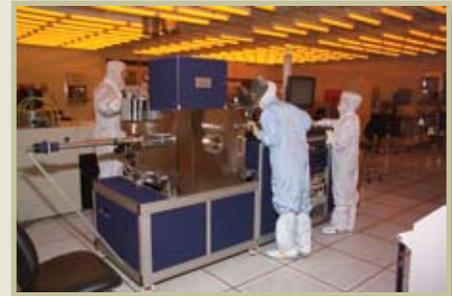
Ion Beam Deposition ▶
