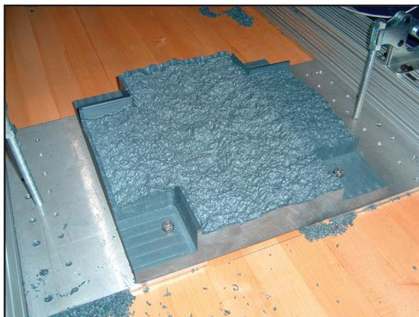
Fabrication of rough surfaces for acoustic analysis.
