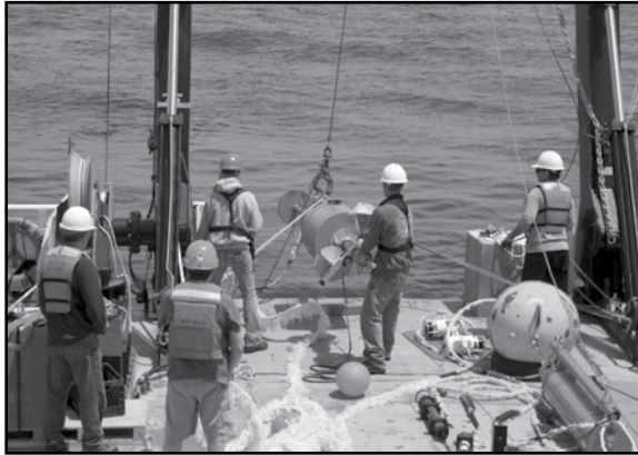
At-sea deployment of underwater acoustic communications source/receiver array. The purpose is to conduct multiple-input-multiple-output (MIMO) underwater acoustic communications experiments to increase the bandwidth for distributed systems.
