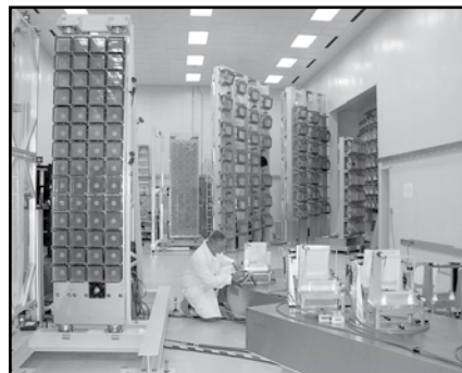
Nike is the world's largest krypton fluoride (KrF) laser and is used to explore physics issues for laser fusion. Shown is the propagation bay where 56 short-duration (4-5 ns) beams are directed by mirrors first to the electron-beam-pumped amplifiers and then to the target facility. The Nike KrF system achieves extremely uniform high-intensity illumination of planar targets by overlapping numerous smoothed laser beams. Typical experiments include studies of the ablative acceleration of matter to high velocities (100 km/sec) and studies of the reaction of materials to very high pressures (10 million atmospheres) produced by the laser light.
