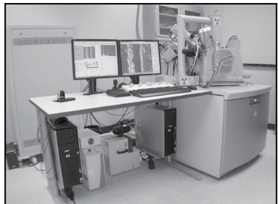
Environmental scanning electron microscope with focused ion beam (ESEM/FIB) coupled with an energy dispersive X-ray detector.
