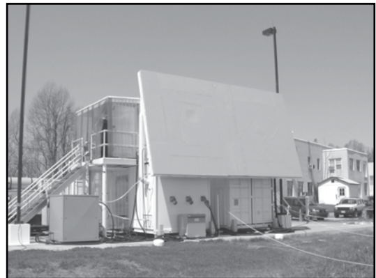
The Advanced Multifunction RF Concept (AMRFC) test bed is a proof-of-principle demonstration system capable of simultaneously transmitting and receiving multiple beams from common transmit and receive array antennas for radar, electronic warfare, and communications.
