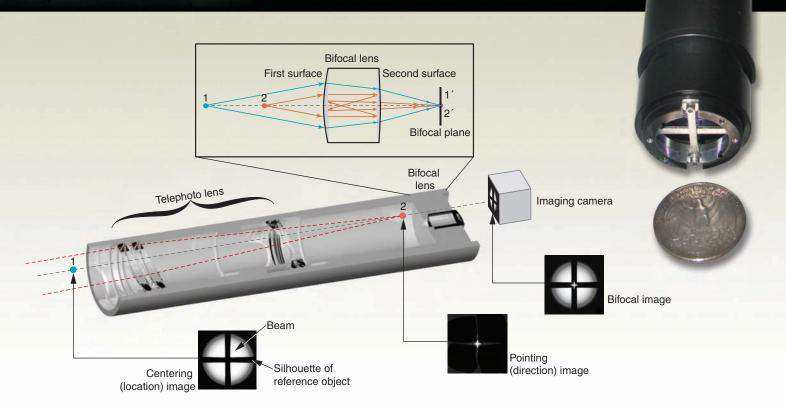
The laser beam centering and pointing system combines two laser beam alignment sensors—centering and pointing into one. The dual-imaging bifocal lens images both the "centering" and "pointing" data onto the camera.
