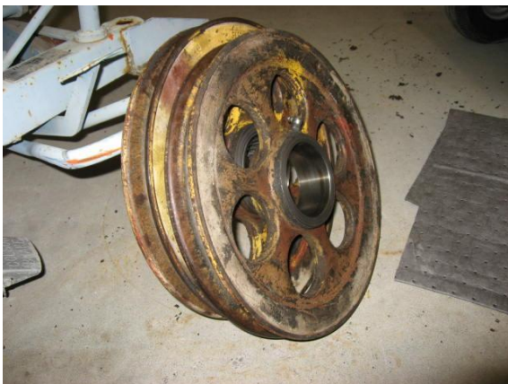
Dismantling and cleaning of the hook block from mobile crane 17T-05690 in preparation for new bearings
