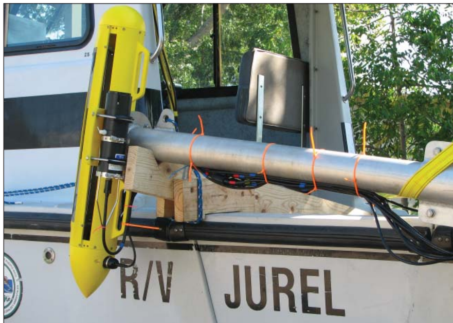
Figure 2.38. The Teledyne Benthos C3D (200 kHz) LPM PDBS was pole-mounted on the R/V Jurel . This system was used to collect bathymetry and intensity imagery in Jobos Bay. Photo: NOAA CCMA.
