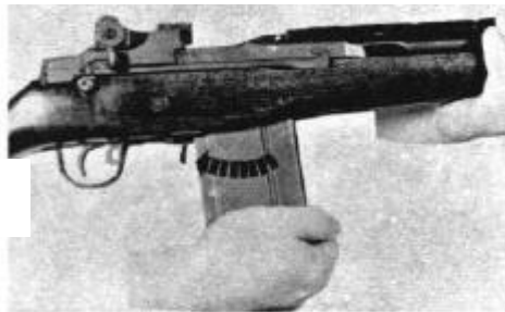
Figure 4.2.1. Loading magazine into rifle, step two.
