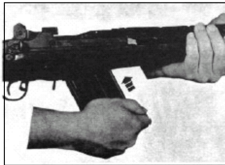
Figure 4.2. Loading magazine into rifle, step one.
