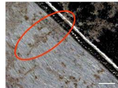
Non-Treated surface (SCC occurrence)
