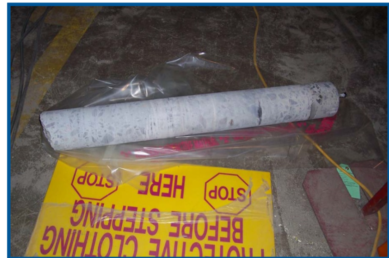
Concrete Core Sample
