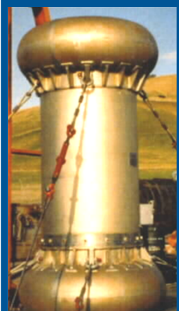
Cask: GE-2000 Owner: GE/DOE Max. Capacity: 42 MTR, 1 HFIR Core Fleet size: 3: 2 (GE), 1 (DOE)
