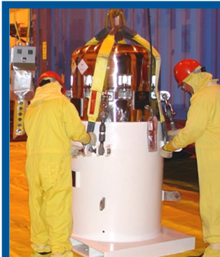
Cask: JRF-90Y-950K Owner: JAERI Max. Capacity: 5 MTR Fleet size: 4
