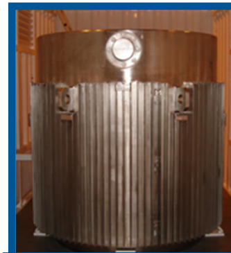
Cask: TN-MTR Owner: Cogema Logistics Max. Capacity: 52 MTR, 52 DIDO Fleet size: 3
