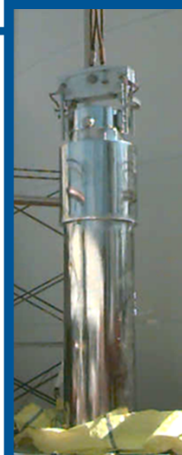
Cask: LWT Owner: NAC Max. Capacity: 42 MTR Fleet size: 5
