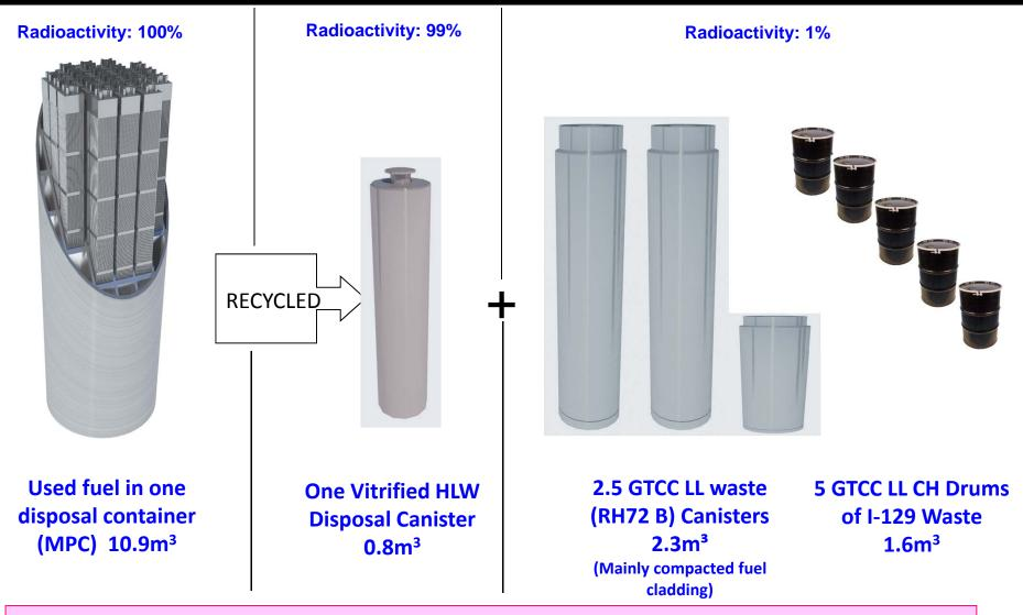
Vitrified product volume reduction from SNF is here shown to be about 13-fold. This allows for vitrified product containers Depending on heat-related packing factors that are assumed, this factor can fall to about 6-fold
