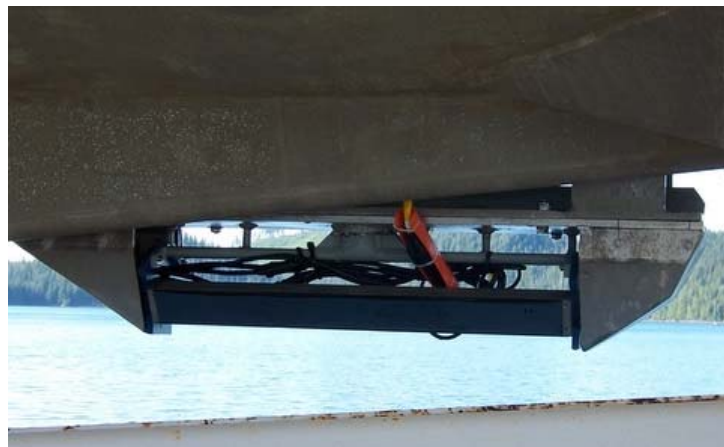
The C3D sonar transducer on the hull of the #6 Launch.
