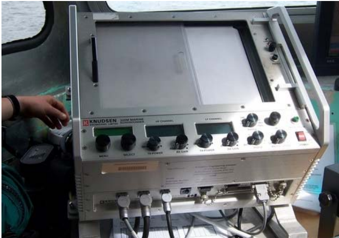
This is the Echosounder machine that records the data from the single beam transducer.
