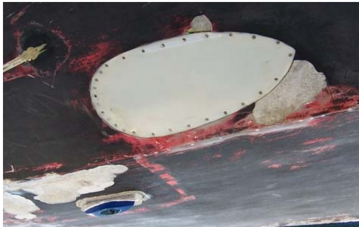
This is a single beam transducer on the hull of launch #1. The small blue oval on the hull is a "fish finder" or depth sounder.
