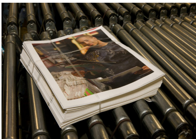
Figure 20: Bundle Tied with Plastic String on Rollers
