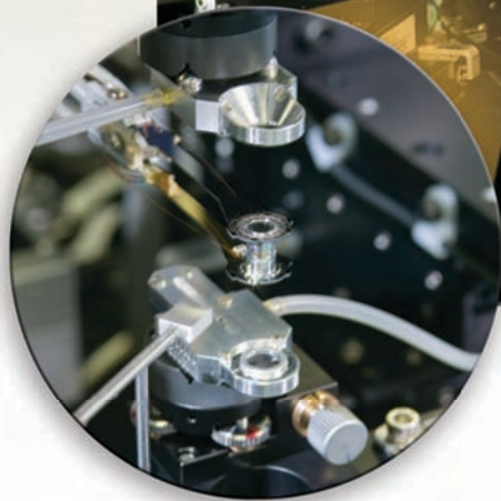
Systems engineer Richard Montesanti operates the precision robotic assembly machine. The inset shows an assembled fusion ignition target.
