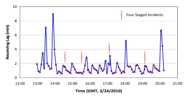
Figure 5. Time lag in receiving messages during the road test of the truck
