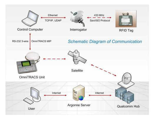
Figure 2. Schematic diagram of communication paths between the ARG-US RFID equipment and OmniTRACS satellite communication gear of Qualcomm/TRANSCOM
