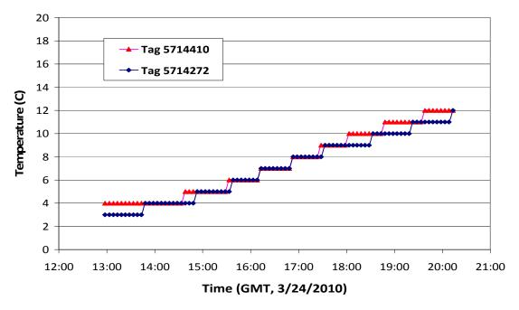
**Figure 6.** Temperature data from two of the tags in the truck during the road test. The gradual increase in temperature occurred because the test started at ≈8 am local time.
