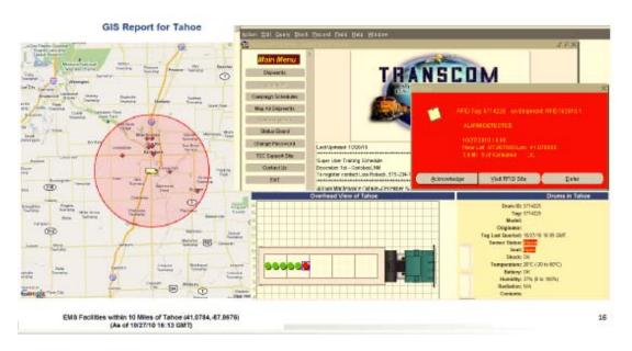
Figure 8. Screens appearing after alarm detected in the TRANSCOM/ARG-US RFID system
