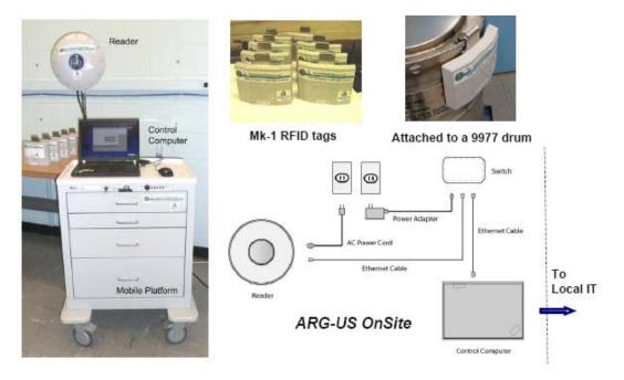
Figure 1. An ARG-US system on wheels, demonstrating system mobility.
