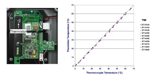
Figure 3. Calibration of tag thermistors versus certified thermocouples.
