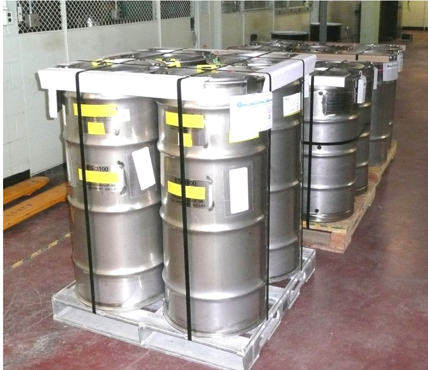
FIGURE 2 Banded ES-3100, 9977, and 9975 Drums on Three Pallets Ready for the DEMO.
