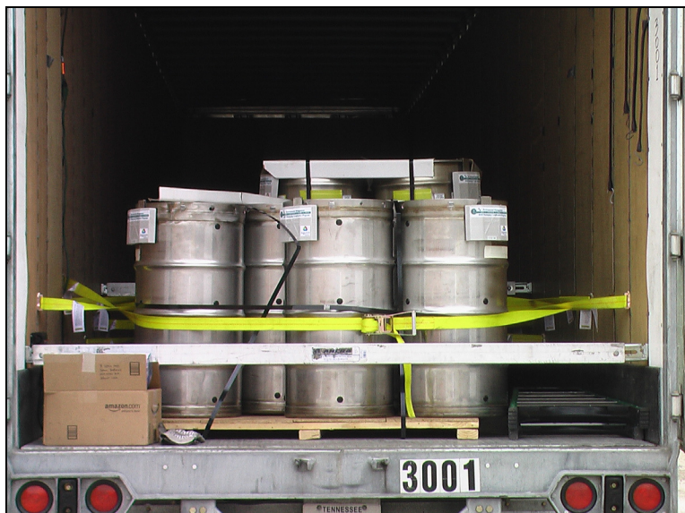
FIGURE 14 The Bandings Holding the Five 9977 Drums. Because the bandings had worked loose during the transport, the drums moved laterally on the pallet and caused a shock sensor alarm.
