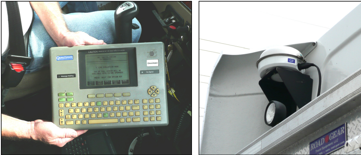
FIGURE 10 TRANSCOM Tracking System — Tablet Terminal (left) and Externally Mounted Antenna (right). GeoLogic Solutions tracking system (not shown) has a nearly identical setup.
