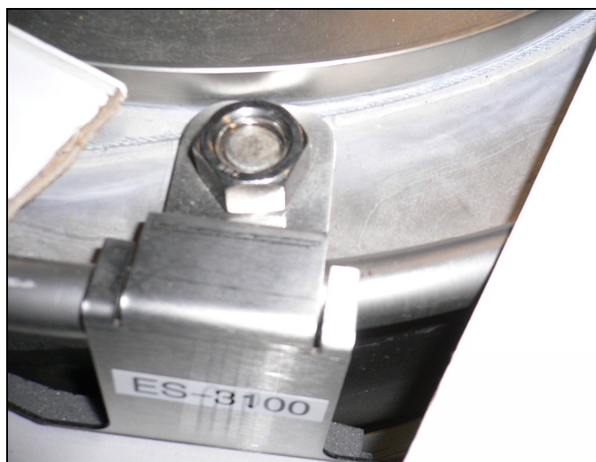
FIGURE 15 Drum with Bumped Tag. This tag was apparently bumped during unloading, which resulted in a slightly twisted bracket. A seal-sensor alarm resulted from this event. The seal sensor was undamaged.
