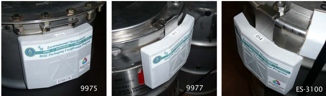
Figure 1. Mk-1 tags bolted to Model 9975, 9977, and ES-3100 packaging.
