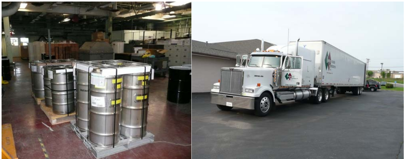
Figure 5. DEMO packages (Model ES-3100, 9977, and 9975) fitted with RFID tags on pallets waiting to be loaded onto the tractor-trailer.
