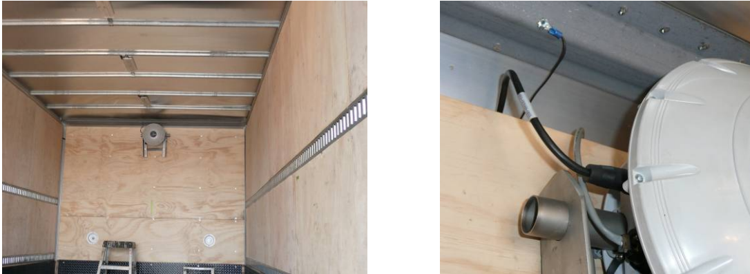
FIGURE 5 Mounted RFID Fixed Reader on the Forward Wall of the Trailer
