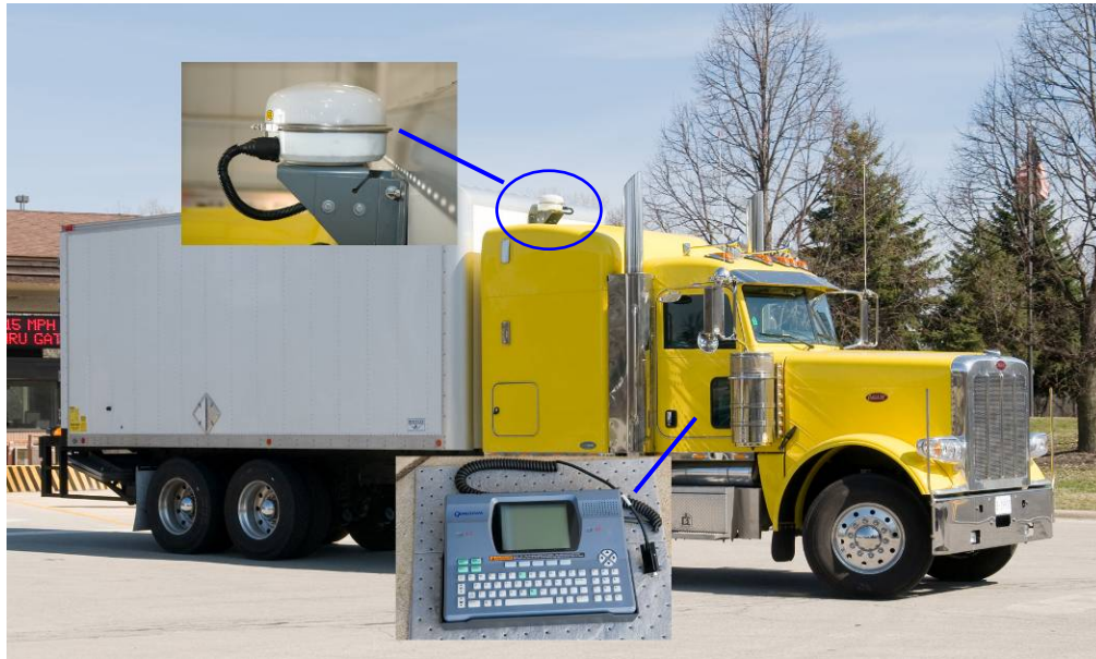
FIGURE 4 “Big Bird” with the Externally Mounted Transponder and the Tablet Communication Terminal in the Cab
