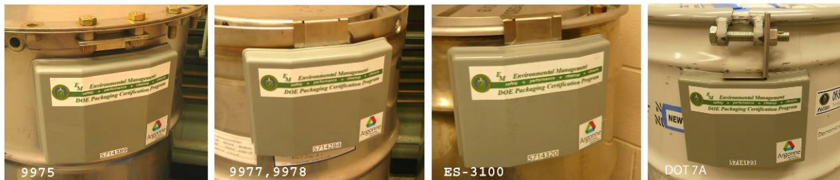
FIGURE 3 ARG-US MK-II RFID Tag (top) and Mounting on Different Drum Types (bottom, from left to right: 9975, 9977/9978, ES-3100, DOT 7A)
