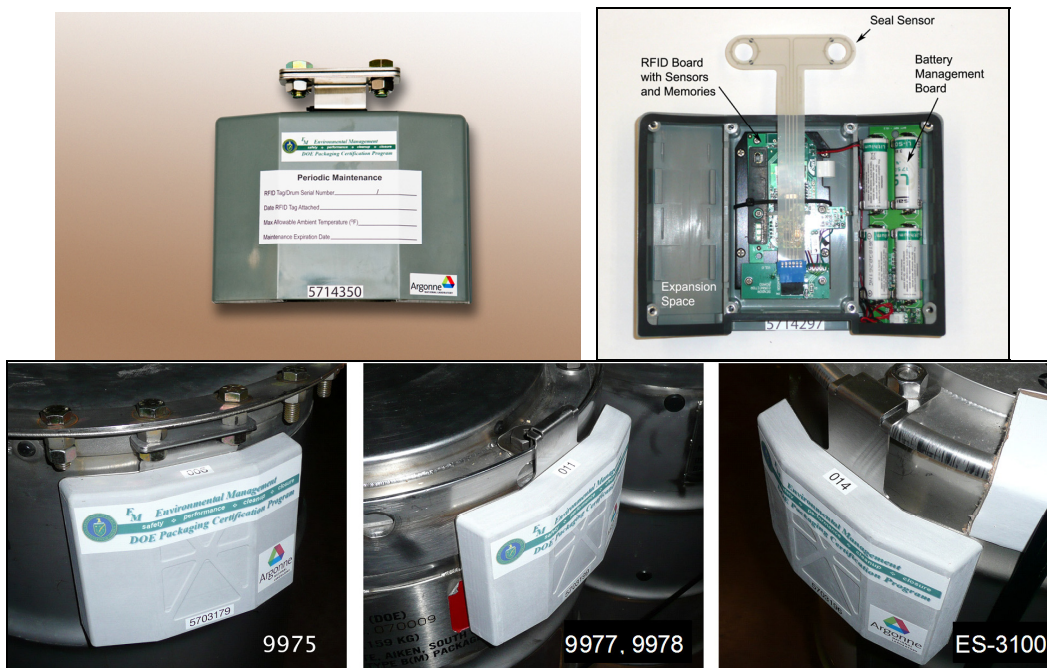
FIGURE 3 Mk-II RFID tag (top) and mounting of the tags on multiple drum types.
