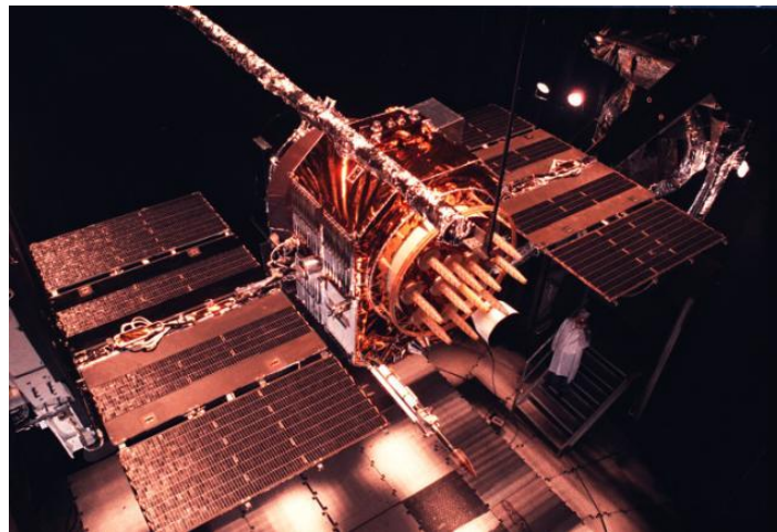
A Global Positioning System Satellite Block II test in the Mark 1 space chamber, 1985.
