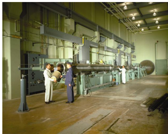
Taken in 1963, this photo shows the two-stage launcher for the 1,000-foot hyperballistic Range G which uses black powder, a piston and compressed hydrogen gas to propel models velocities up to and exceeding Mach 29.
