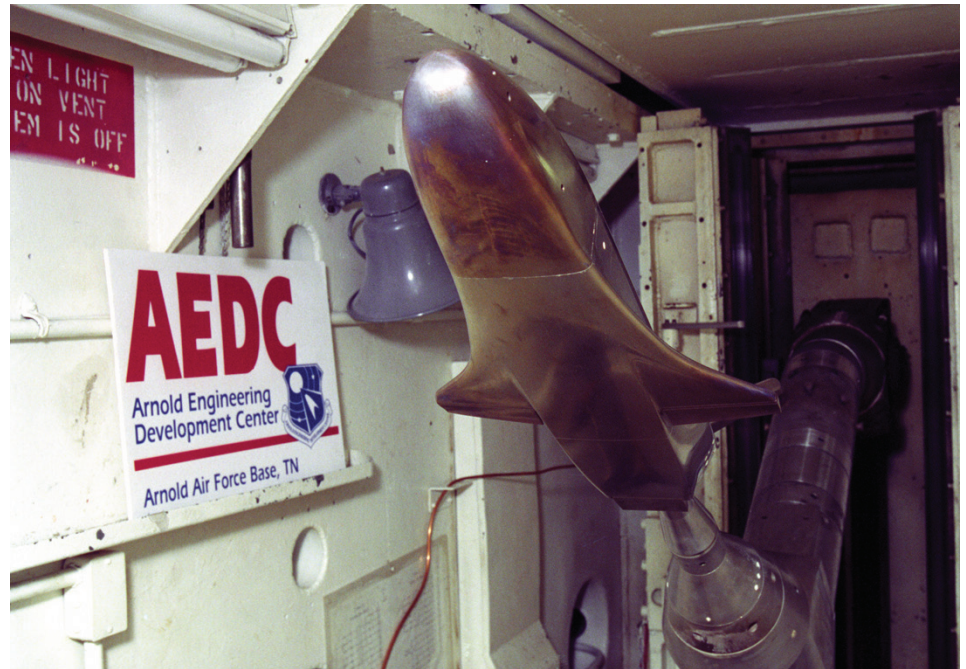
A 2001 wind tunnel test in VKF used a 6-percent scale model of Boeing's X-37 to investigate the aerodynamic forces. (AEDC file photo)
