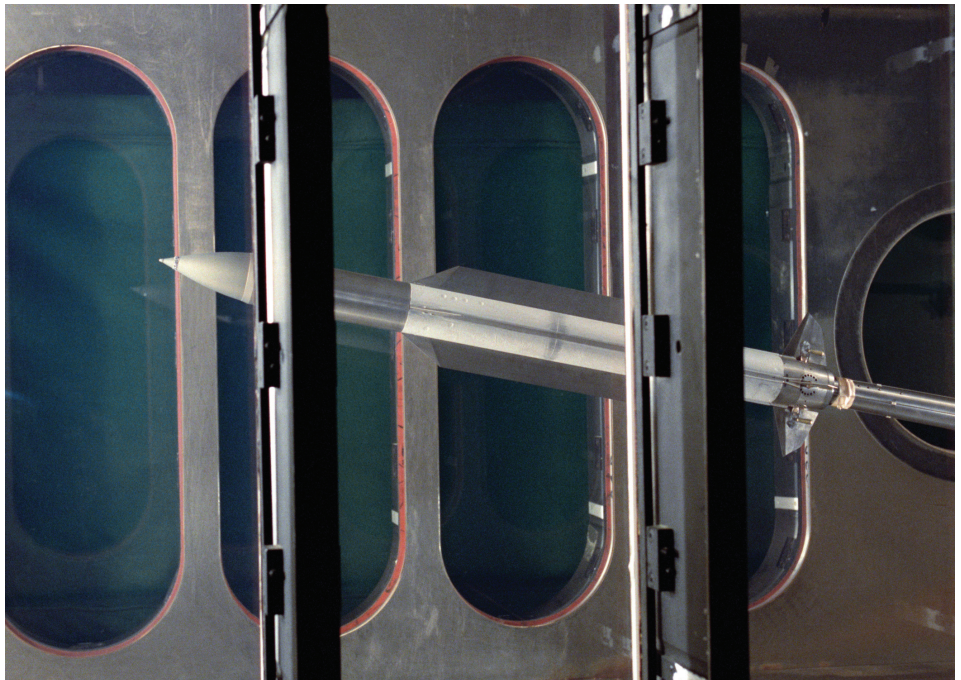
Flight simulation testing was conducted on the Navy Standard Missile in VKF Tunnel A in 1994 at AEDC. (AEDC file photo)
