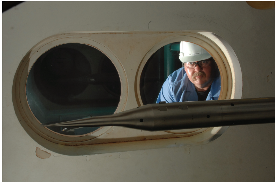
Joe Syler, Tunnel B operations crew member, looks on as a model of the NASA Hypersonic Boundary Layer Transition (HyBoLT) rocket is prepared for testing in 2007 at Mach numbers of 6 and 8 in the von Karman Gas Dynamics Facility’s Tunnel B. (Photo by David Housch)
