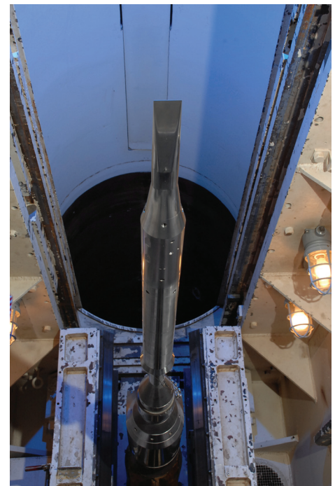
In 2007, a NASA hypersonic boundary layer transition (HyBoLT) rocket model underwent testing in Arnold Engineering Development Center's von Karman Gas Dynamics Facility's Tunnel B. (Photo by David Housch)
