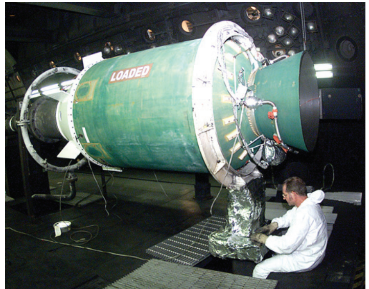
AEDC Outside Machinist J.R. Durham prepares a Minuteman Stage 3 motor before testing in J-6 in 2003. Operators fired the randomly selected motor at a simulated altitude of 100,000 feet to qualify the motor's production lot. (AEDC file photo)
