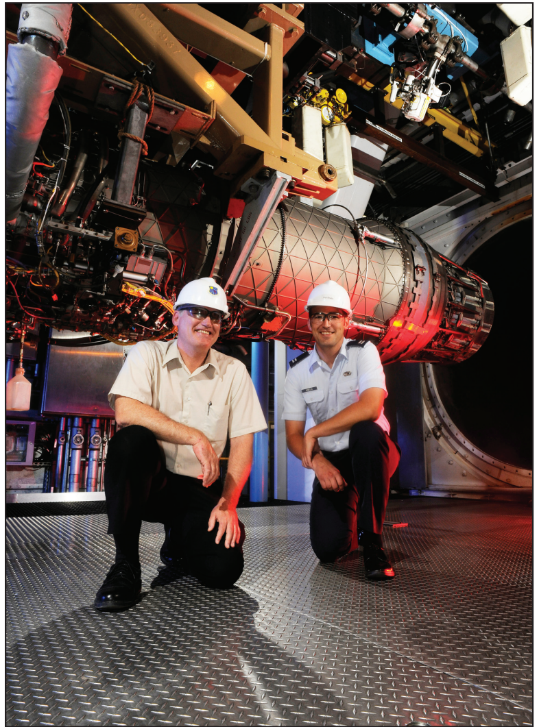
ATA project manager Tom Schmidt, left, and turbine engine test project manager Capt. Scott Rinella pose in front of an F100-PW-229 engine in the Engine Test Facility's SL-3 test cell. The engine, which is used in the F-15 Eagle and F-16 Fighting Falcon, underwent an 11-month Component Improvement Performance test to increase the lifetime of the engine. (Photo by Rick Goodfriend)
