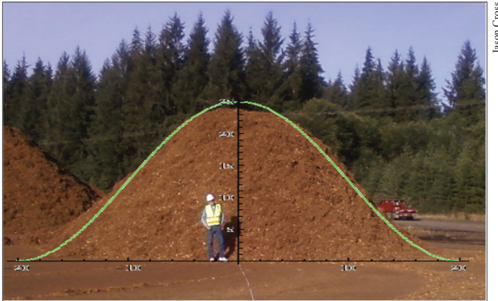
Figure 5—Processed hog fuel pile with profile curve estimate. The function describing the curve (in green) is given by the equation: y = \{[\text{Cos}((\pi \times x) \div r) + 1] \div 2\} \times h . Where r is the half-period of the curve ( y -axis to endpoint) and was derived from a direct measurement of circumference; h was the height measured from 100 distance from the center using a clinometer.
